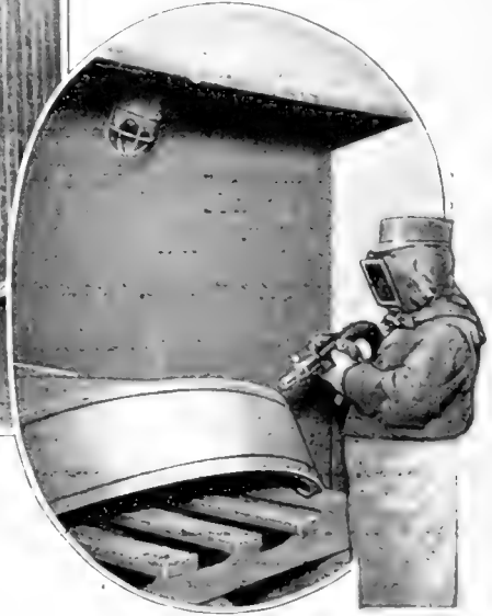
The Head-Dress Allows a Free Passage of Air About the Head and Through the Fine Copper Gauze Which Protects the Eyes: The Hands Are Heavily Gloved
